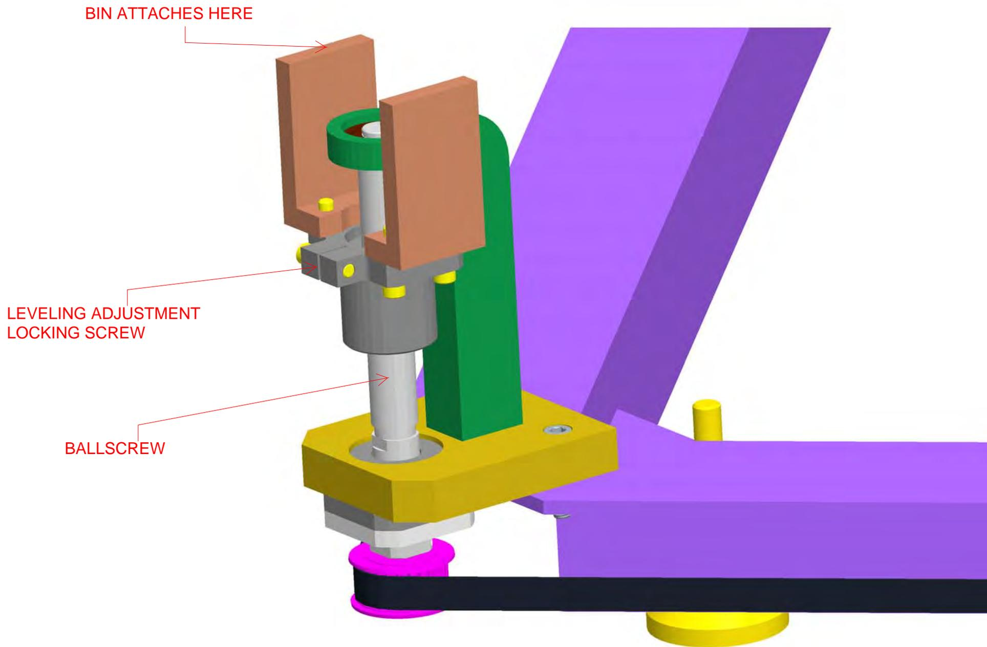
LIFTING MECHANISM DETAIL
