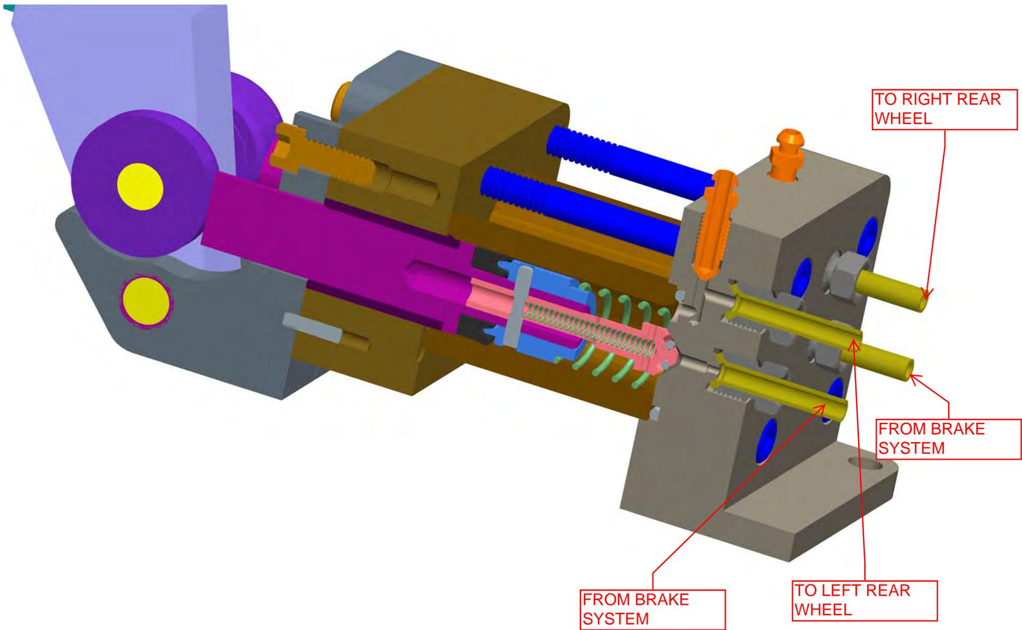
O-RING ISOLATES WHEEL FROM BRAKE SYSTEM AFTER .026" OF PISTON TRAVEL
